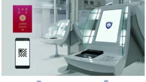
Passengers are able to make customs declarations electronically by holding your passport and 2D code on the scanner of electronic declaration terminal.
