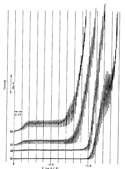
Fig.2 - (3) Polarogram of hydrogen catalytic wave by \text{Rh}_2(\text{SO}_4)_3 in N - HCl.
