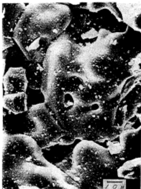
Photo.11 Sintered alumina (1,700 °C) ( \times 1,000 )
