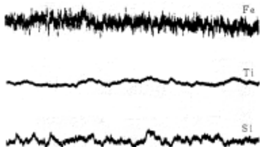
Fig.4 Artificial emery by X - ray microanalyser (5,000cps)
