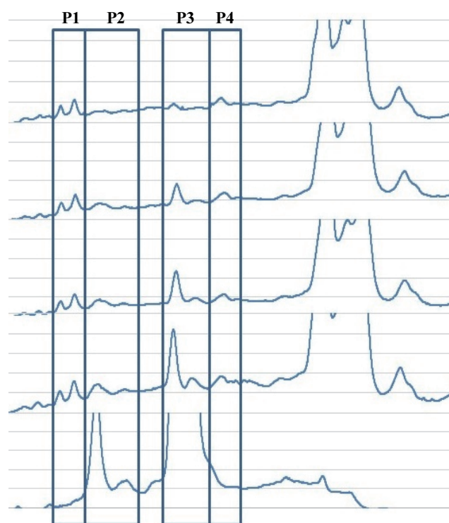
Fig. 10 CE electropherograms of milk protein mixtures (Expanded Fig. 9; migration time, approx. from 13 min. to 20 min.)
