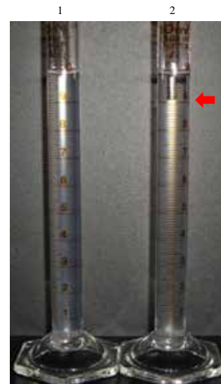
Fig.12 Sedimentation of corn starches by using potassium iodide (30 g KI/ 100 ml H 2 O)
