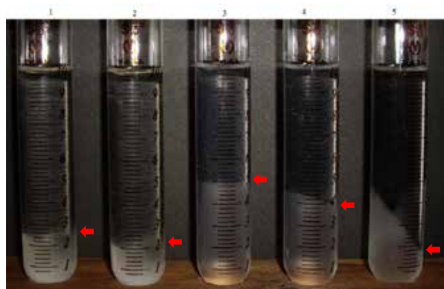
Fig. 20 Sedimentation of corn starches by using sodium hydroxide (0.1 g NaOH/100 ml H 2 O) and a centrifuge
