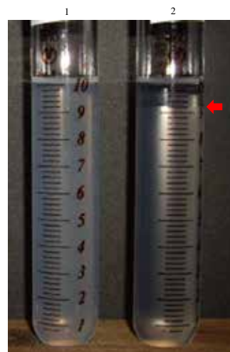
Fig.16 Sedimentation of corn starches by using potassium iodide (30 g KI/ 100 ml H 2 O) and a centrifuge
