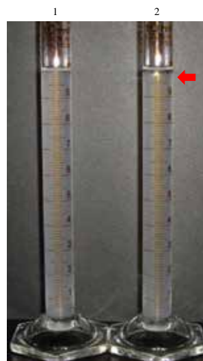
Fig.14 Sedimentation of rice starches by using potassium iodide (30 g KI/ 100 ml H 2 O)
