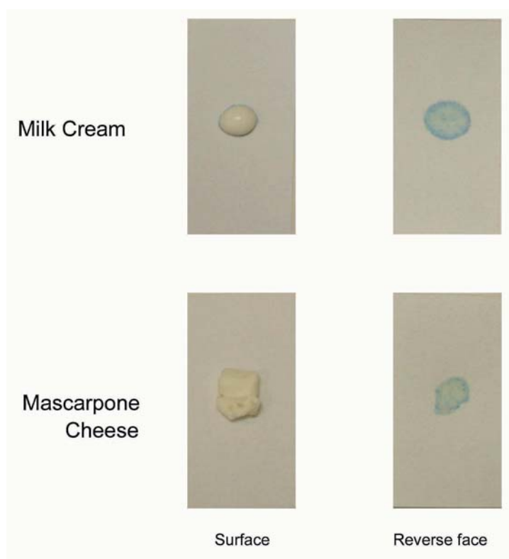
Fig. 2 Coloration of Water Detection Paper caused by milk cream and mascarpone cheese.
