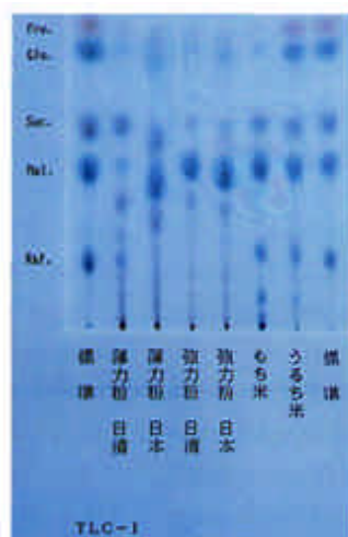
Photo 1 TLC Pattern of Sugars in Wheat and Rice Flours
