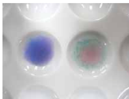
Fig. 1 Color by ketamine test written on paper (left: ketamine HCl, right: blank)
