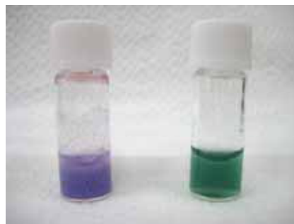
Fig. 2 Color by ketamine test by using vial (left: ketamine HCl, right: blank)
