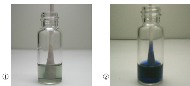
① 0.5% Ascorbic acid solution, ② 0.5% Methamphetamine solution. (3 minutes later after addition of samples)
