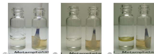
① Conc Hydrochloric acid ② Conc Sulfuric acid ③ Glacial Acetic acid (Photos of 3 minutes. Left: Narcotic reagent Right: Stimulant reagent)
