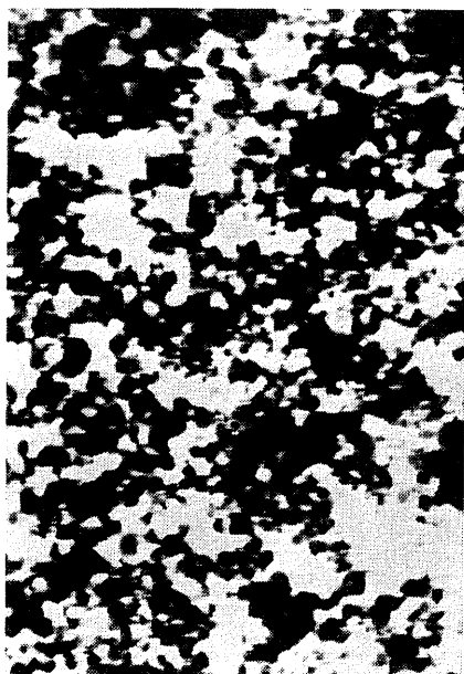
Photo.9 Acrylonitril styrene butadiene Copolymer (X2,000)
