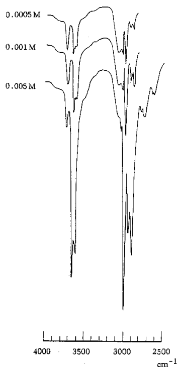
Fig.10. Infrared spectra of 2,3-butanediol (C Cl 4 soln. 20mm KBr cell M=mol)
