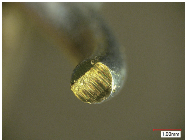
Photo 1 Observation of section of gold products coated with rhodium.
