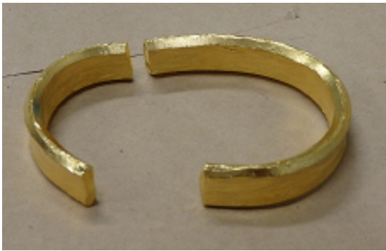
Photo 2 A gold product, divided by a metal-scissors cutting, whose plating had previously been removed
