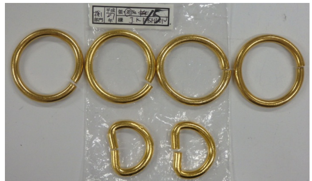
Photo 5 Samples of lifting hooks for handbag, whose coating materials were removed with dilute nitric acid aqueous solution
