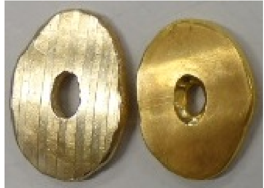
Photo 4 Examples of coin-like gold products whose coating materials were removed with dilute nitric acid aqueous solution
