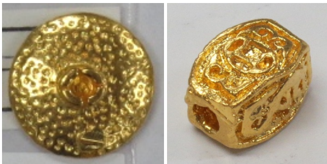
Photo 1 Concavo - convex gold artifacts with or without holes after removal of their plating
