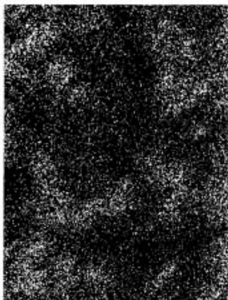
Photo. 11 Cobalt contained in cermet by XMA ( \times 5,000 )
