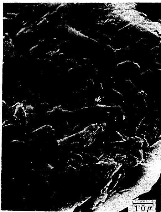
Photo. 6 Crystalline graphite ( \times 1,000 )
