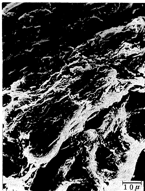
Photo. 14 Artificial graphite (Powders) ( \times 1,000 )
