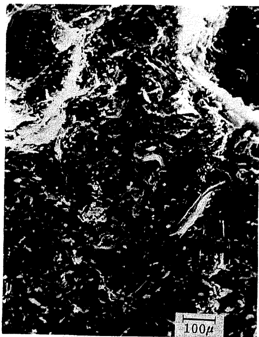
Photo. 7 Calcined graphite ( \times 100 )
