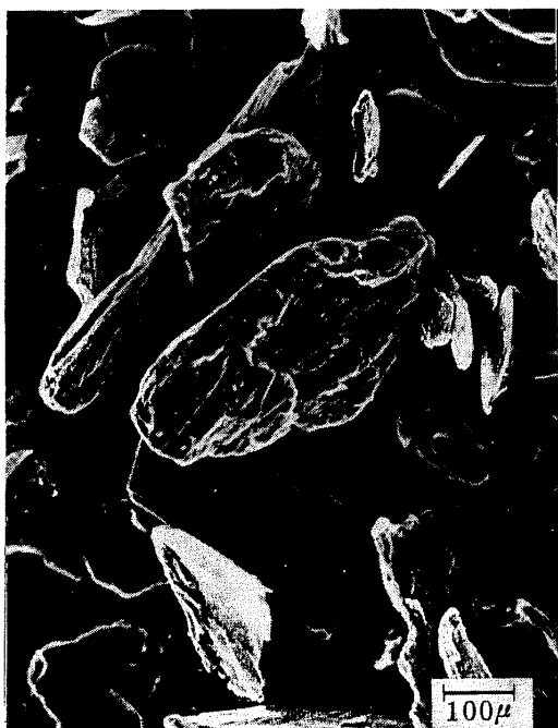
Photo. 5 Crystalline graphite ( \times 100 )
