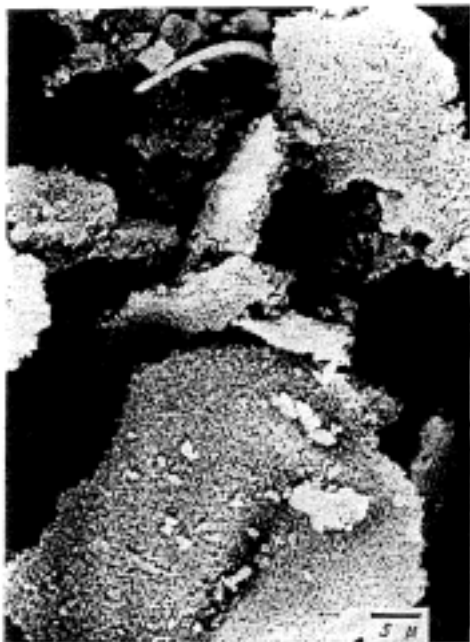
Photo.9 Aluminium oxide ( \times 2,000 )
