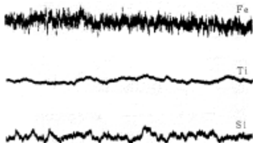
Fig.4 Artificial emery by X - ray microanalyser (5,000cps)
