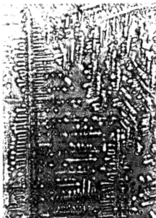
Fig.8 Photomicrograph of dendrite structure of "Jade Qual"
