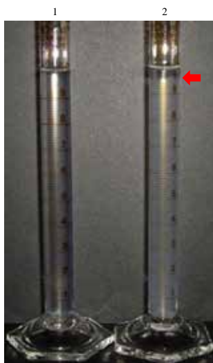
Fig.13 Sedimentation of potato starches by using potassium iodide (30 g KI/ 100 ml H 2 O)
