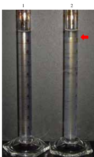
Fig.11 Sedimentation of wheat starches by using potassium iodide (30 g KI/ 100 ml H 2 O)
