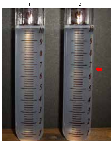
Fig.15 Sedimentation of wheat starches by using potassium iodide (30 g KI/ 100 ml H 2 O) and a centrifuge
