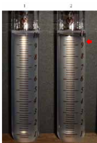
Fig.17 Sedimentation of potato starches by using potassium iodide (30 g KI/ 100 ml H 2 O) and a centrifuge
