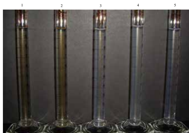
Fig. 21 Sedimentation of wheat starches by using sodium hydroxide (1 g NaOH/100 ml H 2 O)
