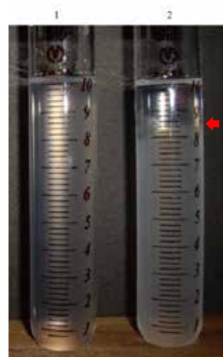
Fig.18 Sedimentation of rice starches by using potassium iodide (30 g KI/ 100 ml H 2 O) and a centrifuge
