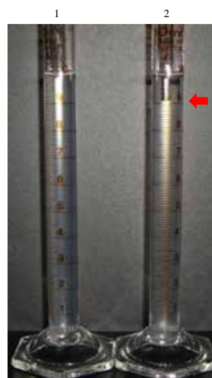
Fig.12 Sedimentation of corn starches by using potassium iodide (30 g KI/ 100 ml H 2 O)
