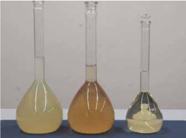
Photo.3 Effect of pretreatment on the color of dextrin roasted starch suspension (2% w/v in water) Left: non-treatment; Center: Solution after neutralization and heating; Right: Supernatant liquid after one-day standing
