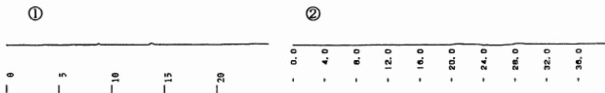
Fig.2 High Performance Liquid Chromatogram of sulfuric acid was neutralized by barium hydroxide
