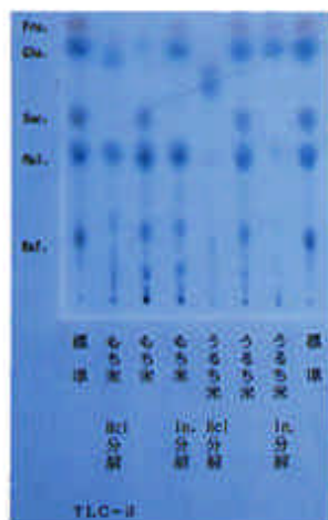
Photo 3 TLC Pattern of Sugars in Rice Flours after Decomposing by Hydrochloride and Invertase
