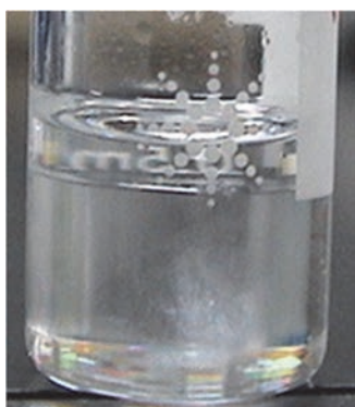
Fig.9 Photo of two-phase separation of TMS-PZ when 10% GHB-Na solution was added.
