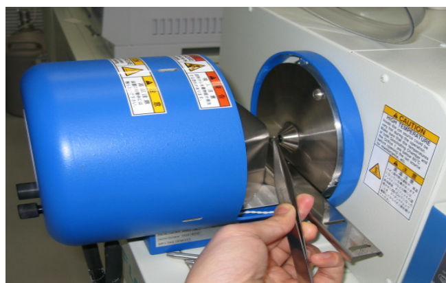
Fig.1 Method of introduction to DART-TOFMS (Tablet method)
