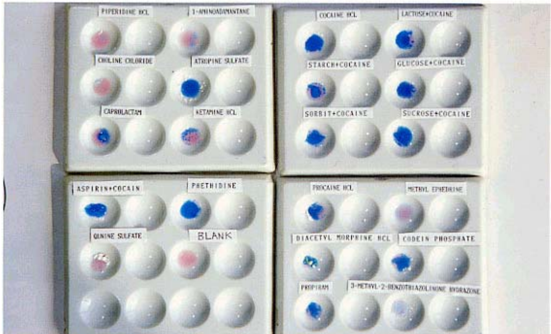
Photo No.3 Cobalt thiocyanate 2% reagent test
