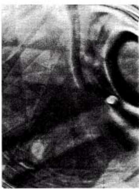
Photo. 8 Crystal border ECP ( \times 100 )
