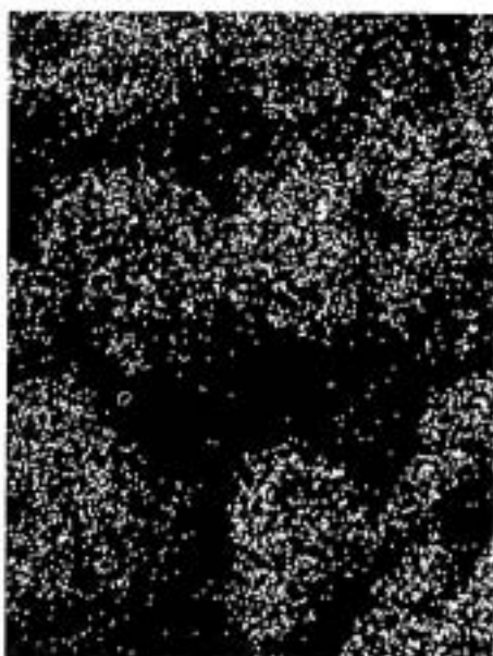
Photo. 4 Nickel contained in alloy by XMA (× 500)
