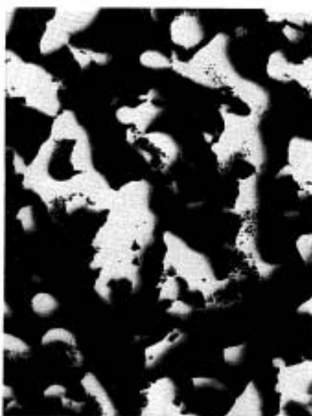
Photo. 6 Observation of cement by SEM (× 3,000)
